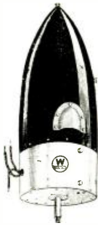
Outside View of Aircraft Generator
