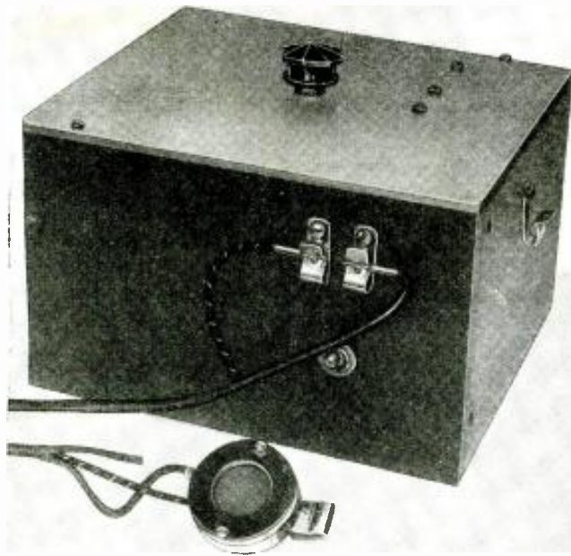
Fig. A Exterior view of the oscillator unit at the "sending" end of the inter-telephone.
